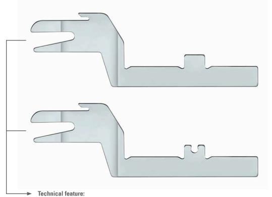
Opening in the front area of the sinker for removal of lint accumulation in the tracks
