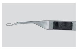
For gauges from E 40, Groz-Beckert has developed and patented a special compound needle with thickened plastic part. The special feature of needle Spec. 51/43.36 G 101 is that its lateral thickened plastic part lends the fine needle adequate stability during loop formation.
